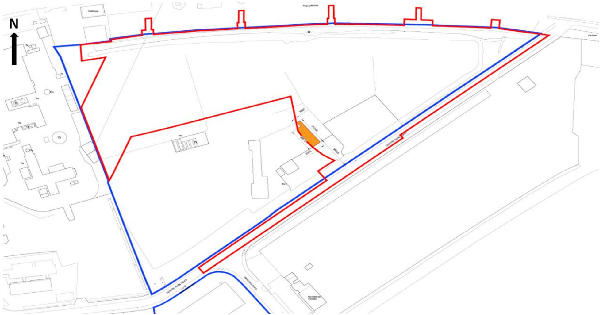
Figure 4: Extract from demolition plan (Drawing No. PE21055-CWO-ZZ-00-DR-A-1002) showing proposed demolition area extent. Orange = demolition areas; Red line = site boundary. Not to scale.
